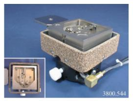
**-45C.544:** Free Furnace Work holder: Cavity Inert Atmosphere, 2X2 Adapter Size, With Dual Mechanical Clamps to Hold a TO-56 Package in Two Different Positions. (1) Horizontal and (2) 7 Degrees From Vertical. 2 x2 Fluoroware Die Presentation.
