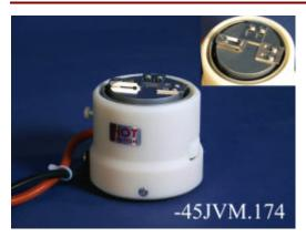
**45JVM.174:** Free Furnace Work holder with Rotating Adapter: Rotating work holder adapter for substrates up to 1.000" x 1.000". Work piece is held by mechanical clamp, with a adjustable backstop and vacuum, with a 1/16" diameter vacuum hole.
