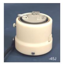
**45J:** Free Furnace Work holder with Rotating Adapter: Basic rotating work holder adapter for substrates up to 1.000" x 1.000". Work piece is held by mechanical clamp, with a adjustable backstop from which many variations are derived:
