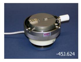
**-45J.624:** Free Furnace with Rotating Adapter: Rotating 3.25" Dia. Adapter: Rotating 3.25" Dia. Adapter with lock open adjustable mechanical clamp and adjustable backstop. Grip range for 0.031 Thick. Substrates 0.125" to 2.500". The Base is Adjustable in height from 2.800" to 3.400".
