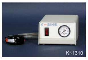
K~1310 Gas Flow Control: The operator, by means of an on/off footswitch, releases the gas to the work area. Immediately after the scrub cycle stops, the footswitch is activated and the die is showered with cool forming gas. A manual adjustment is provided to meter the amount of gas to be released.
