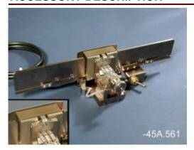
**-45A.561: Free Furnace Work holder**: Non-rotating heated work holder for 3 pin Vertical Lead frames. Work piece is advanced to each bond site manually, then held by 3 clamps, individually adjustable, spring force close & pneumatic open. Assembly No. 3800.561.
