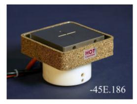
**-45E.186: Free Furnace Work holder:** Non-rotating work holder for substrates 1.250" x 1.250" up to 3.000" x 3.000". Work piece is held by vacuum that has a 1.250" x 1.250" cross pattern, with a .0625" diameter vacuum hole.
