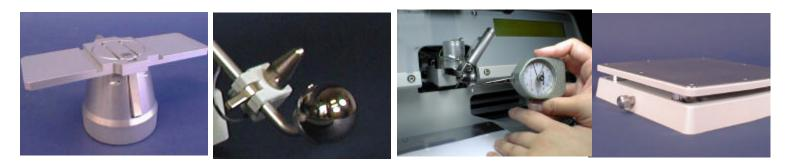
STANDARD SPECIFICATIONS: CONTROL LOGIC: Motorola 68000 Microprocessor MEMORY: 256KB RAM DEVICE STORAGE: Single Device DISPLAY: 40 Character, 4 Line LCD Z-ENCODER RESOLUTION: 0.001" TOOL Z RANGE: 0.625" THROAT DEPTH: 5.25" BOND FORCE RANGE: Adjustable, 5 – 75 grams ESD PROTECTION: Protection against Electrostatic Discharge
